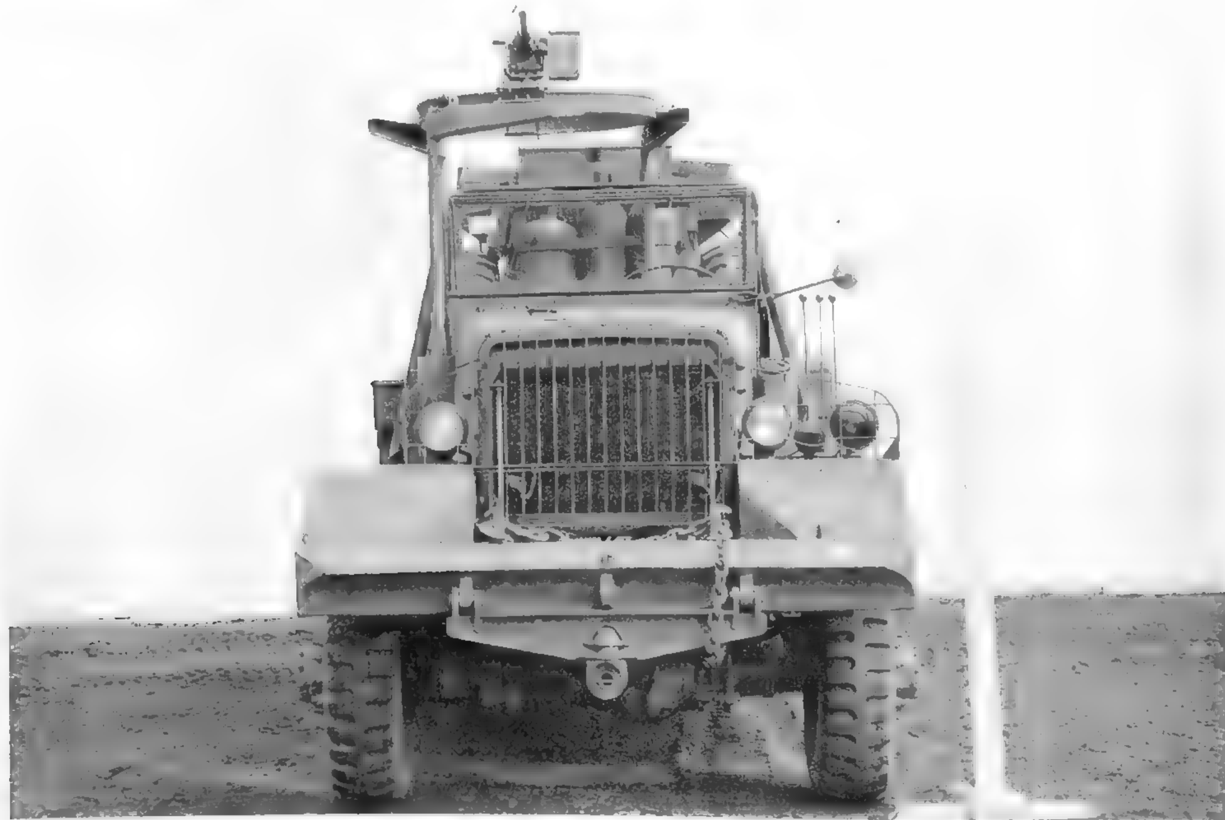
The Series 5 trucks had a very business-like front end. A whiffletree is affixed to the chisel-shaped front bumper, and the two spares, as well as the torch set, are visible through the windshield. This truck is equipped with a ring mount and .50-caliber machine gun, but this was not always the case. (U.S. Army photo)
